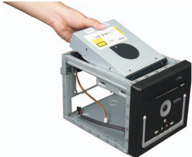
Carefully installing the Asus Blu-ray drive
