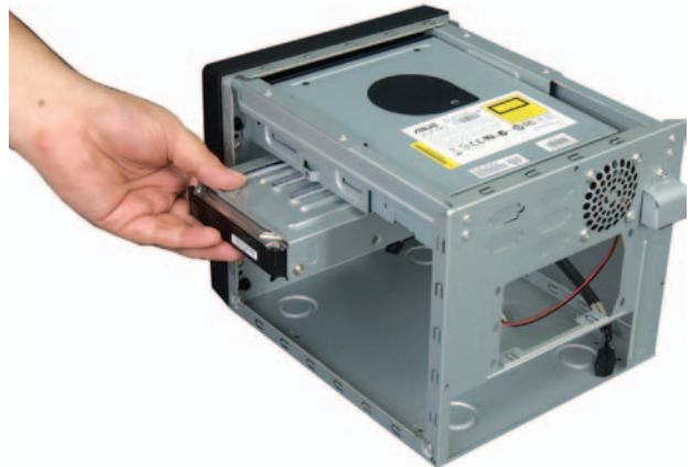
Securing the Hard Drive to the cage and then attaching it to the cabinet
